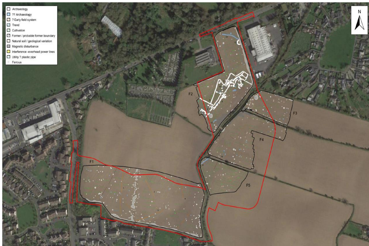
Figure 4.3 Results of geophysical survey carried out within the proposed development area in 2021
